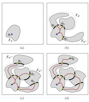
**Fig. 4.** Schematic of a multi-step search. Gray regions are feasible spaces at different stances (a dotted line shows the two components of  $F_{\sigma'}$ ). Bold arcs are intersections between feasible spaces at adjacent stances. Thin lines are one-step motions.
