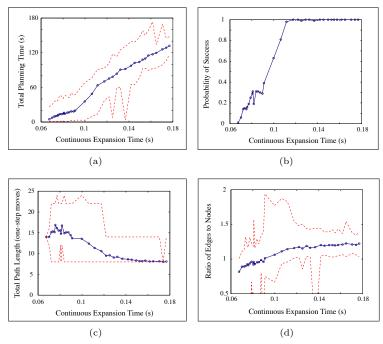
**Fig. 7.** Performance of a basic multi-step search using PRM, as the average time allowed for continuous expansion is varied. Mean values (over many runs) are shown; bounds are dotted lines. (a) Total planning time. (b) Probability of success. (c) Total number of one-step motions in the final path. (d) Ratio of edges to nodes.
