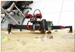
**Fig. 1.** LEMUR IIb, a multi-use robot capable of free-climbing (Mechanical and Robotic Technologies Group, Jet Propulsion Laboratory) [9].
